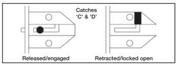
Refer to the tables on page 6, which show the correct catch positions. To extend the ladder, retract left-hand catch 'A' (black) while supporting the front frame of the ladder. Lower the frame slowly until catch 'A' (black) engages again.
