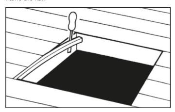
**1.4** Screw hinges (D5) to one edge of the trapdoor using 20mm (3/4") wood screws (D6).
