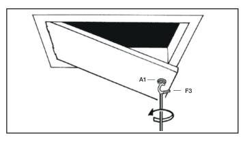
Locate the stowing hook/key (D3) over and at the centre of the REAR ladder section bottom rung and steadily pull the ladder outward and downward until both top stops reach and make contact with the hinge guides.
