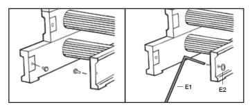
**4.4** Lower 'V' rod to the loft floor, in line with the centre of the ladder.
