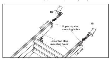
I.2 Slide the hinge guides past both sets of top stop mounting holes, so that the hinge guides are below the top stops, when they are fitted in section 2.
