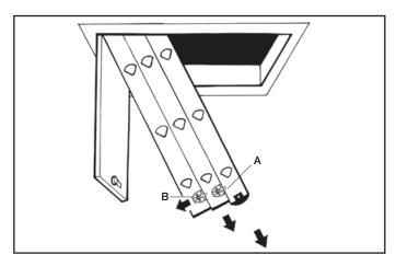
When the ladder has been deployed in accordance with tables on page 6, rotate both right-hand side catch levers downward to unlock and release both catches 'C' and 'D' (blue) and ensure both catches are fully engaged. DO NOT use ladder with any catches ('A', 'B', 'C' or 'D') disengaged. Read the safety labels on the product.
